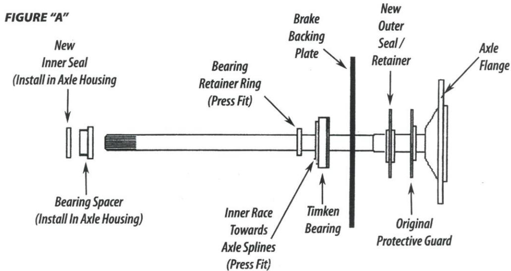
18. Install axle studs and original protective guards. Torque studs to 70 ft/lbs.
